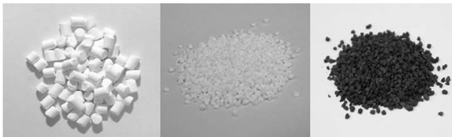
Fig. 1 Alumina pellet, crushed alumina grains, and prepared \text{MnO}_2/\text{Al}_2\text{O}_3 catalyst.
